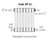
• For TESI radiators lower than 1000 mm or radiators with more than 15 sections.
