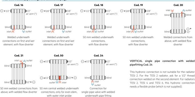
**CAUTION:** these configurations (Cod. 18 and Cod. 19) are not suitable for insertion of the integrated valve (for insertion of the integrated valve, see configurations Cod. 25 and Cod. 26).
