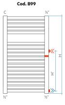
Customised connections (2 pipe fittings + flow diverter)
