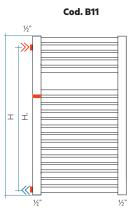
Connections welded laterally in alignment with the first and the last element on the left side
