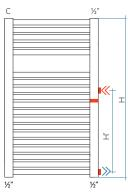
Customised connections (2 pipe fittings + flow diverter)
